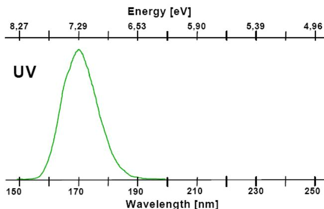
Irradiation with excimer lamps is also suitable for mattifying surfaces such as PVC flooring. At a wavelength of 172 nanometres, these lamps have immensely high-energy emission which starts a polymerization process in the top part of the layer of UV-curable coating. The penetration depth of UV radiation is comparatively low, with the result that this process leaves a micro-folded film on the wet coating without affecting layers deeper down.
